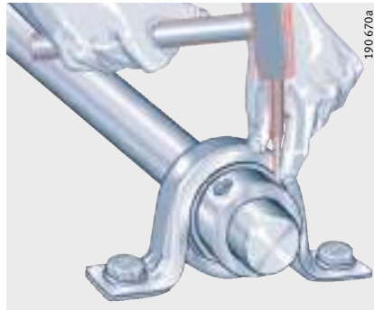
Figure 21 Tensioning the eccentric locking collar
