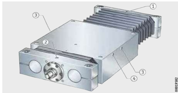
Figure 25 Lubrication points on linear table
